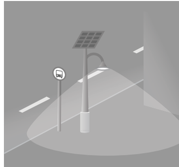
LED-Dimming in Nebenzeiten
